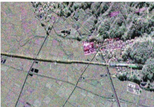
Figure 3: Exit of Joetsu Shinkansen Takiya Tunnel in Nagaoka. Enlarged detail (1.4 km x 1 km) of Figure 1. Shinkansen's elevated railroad runs in the middle of this picture. The derailed train is located to the left.
