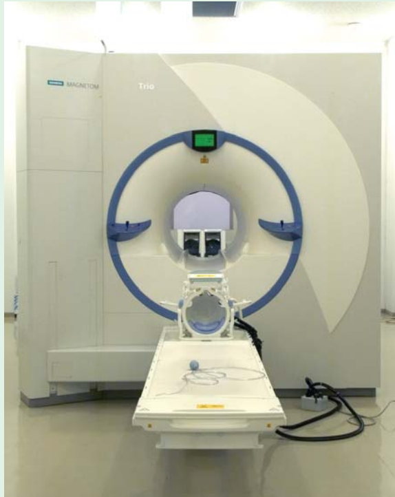
Photo 2-1. The fMRI unit, which generates a high magnetic field of 3.0 Tesla
