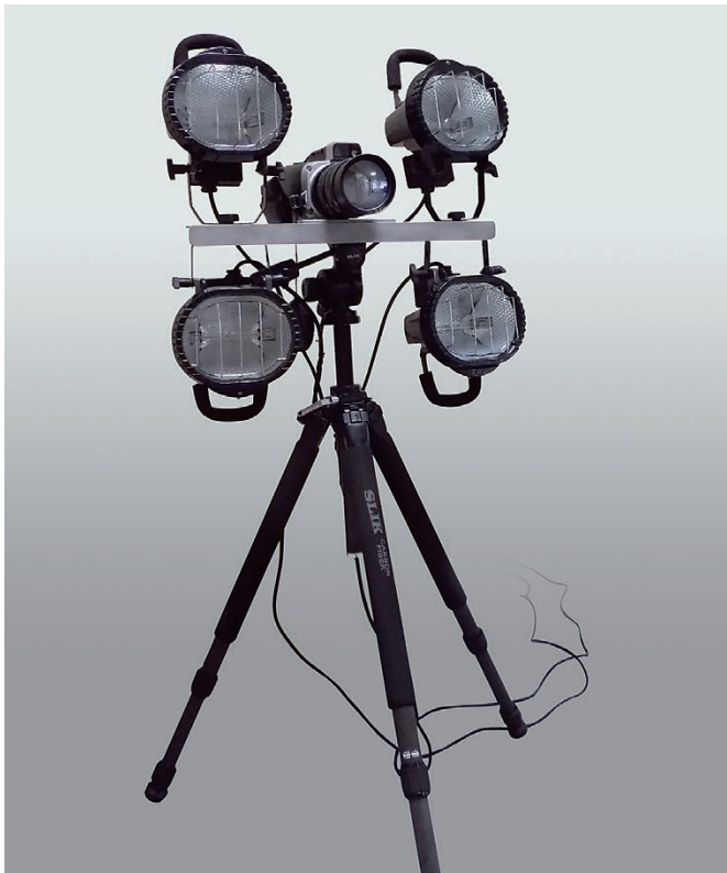
Figure 2 Infrared two-dimensional lock-in amplifier system
