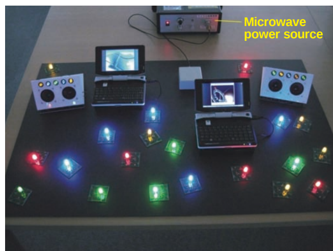
Figure 5●Performance of Contactless Power Transmission to the Small Devices Including Loudspeakers, LED Lights, and Monitors that are Placed on Arbitrary Locations on a Sheet Medium for Communication
